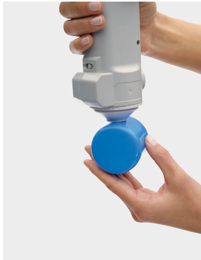
Color measurement of plastic article with spectrophotometer CM-700d (Photo: Konica Minolta)
